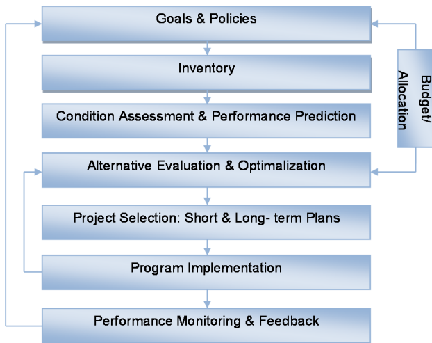
Figure 4 The proposed generic scheme for an asset management system
