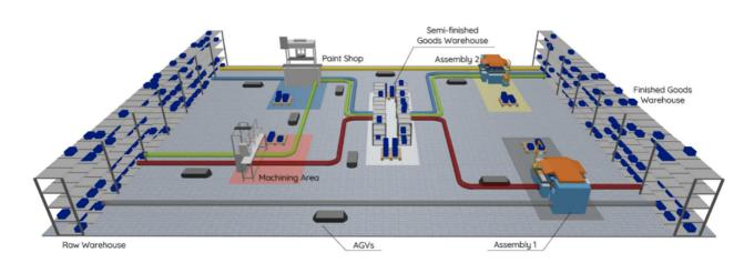
Figure 4 The 3D simulation model of the example factory
