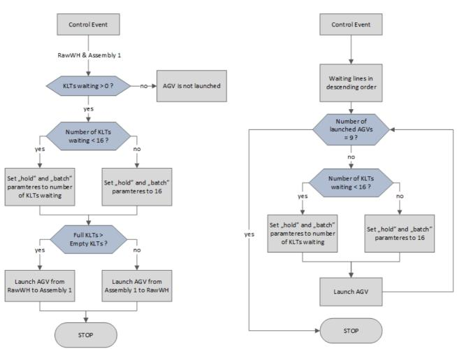
Figure 7 Proccess Chain of traditional (left) and PI-based (right) system
