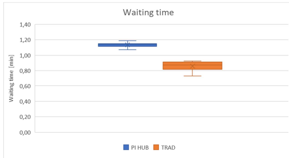
Figure 11 Waiting time of KLTs for PI-based and traditional structures
