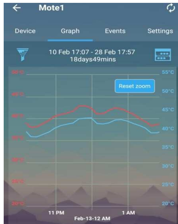
Figure 6 Display of measured operating temperatures of rivet heads over time
