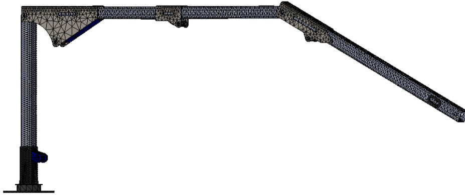
Figure 14 Solidworks mesh modeling of lifting mechanism
