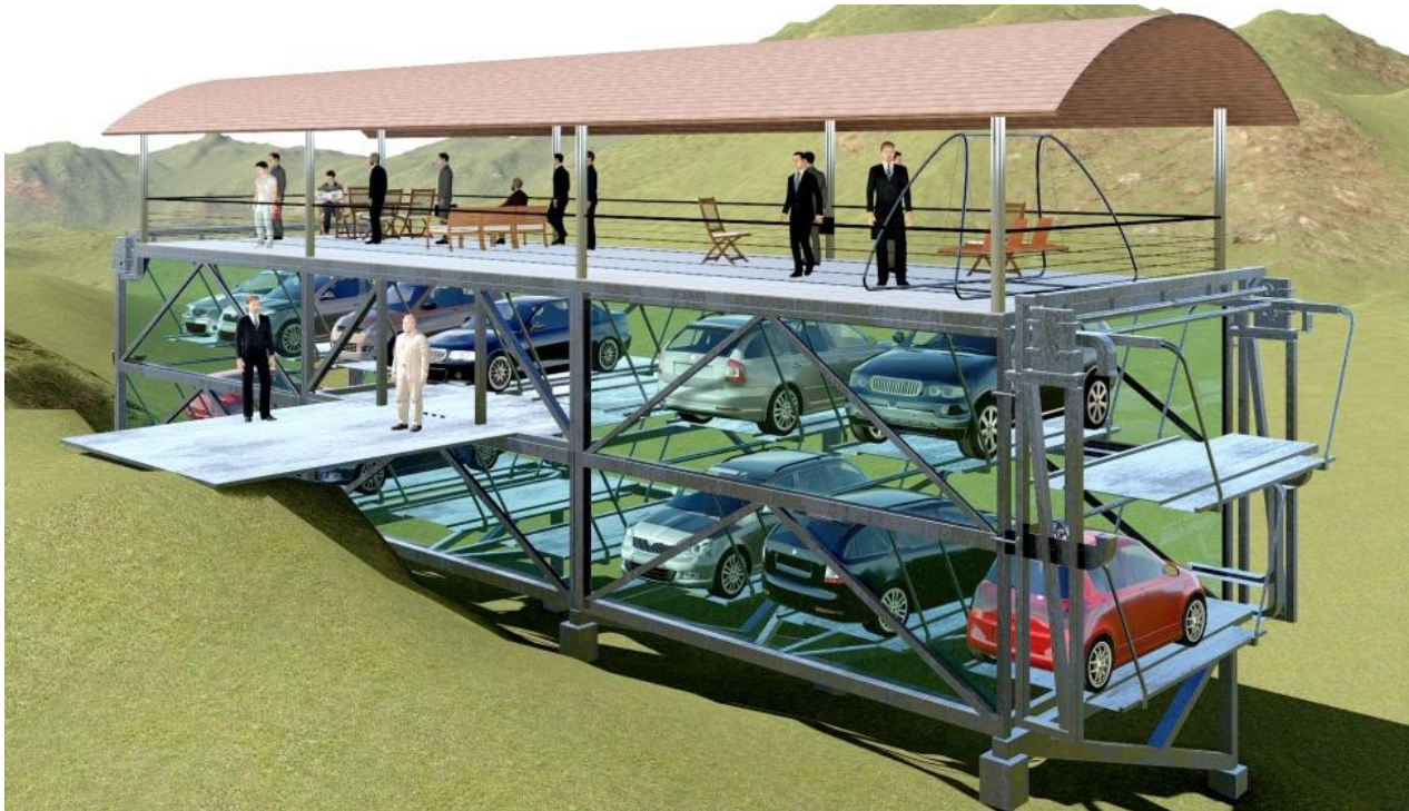
Figure 8 Vertical parking with horizontal vehicle arrangement
