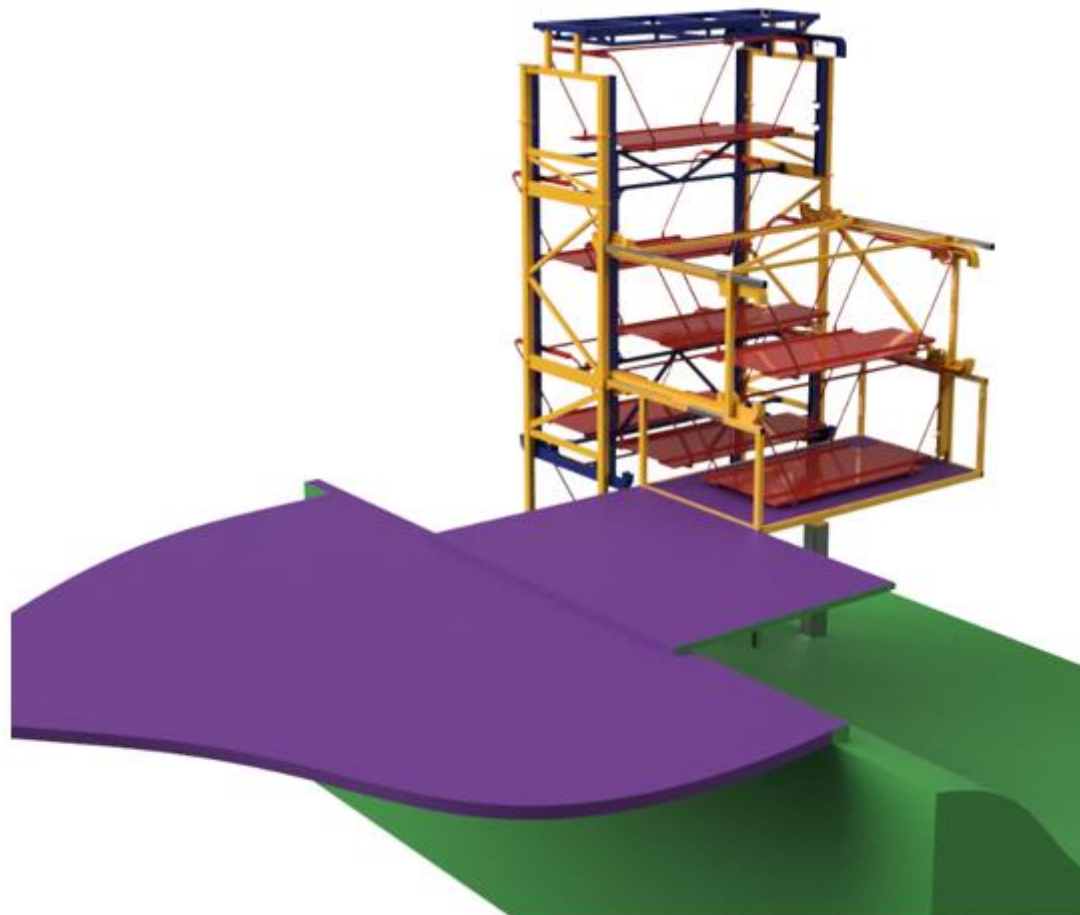
Figure 6 The balcony parking system Mechanized garage with elevator and movable cradles in vertical and horizontal planes
